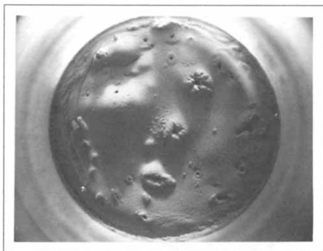
Figure 10. Top view of a test tube after about 1,500 h of settling of a 6.0% by volume \alpha\text{-Fe}_2\text{O}_3 suspension.
